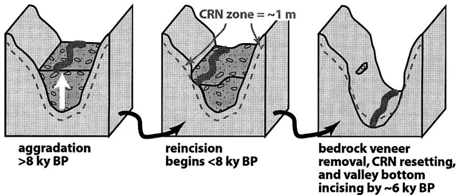
Fig. 10. Schematic drawing of cosmogenic radionuclide (CRN) resetting in Marsyandi's Greater Himalayan reach. River valley aggrades with alluvial fill  $>8$  ky BP. Between 8 and 6 ky BP, the alluvium and a bedrock veneer  $\geq 1$  m thick are removed from the valley, resetting the surface rock's CRN concentration to zero. Fragments of fluvial deposits support the idea that alluvium reached  $>100$  m above the modern river level.
